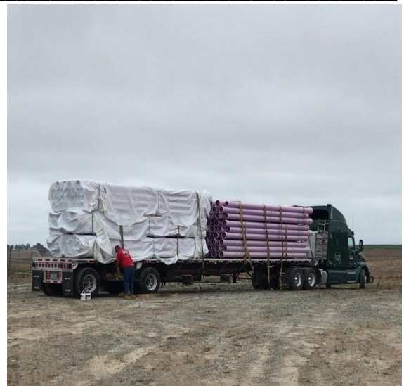
Delivery of "purple pipe" for recycled water
